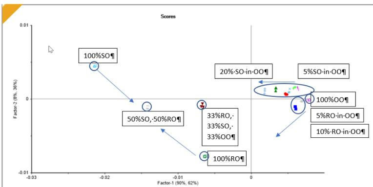
**Figure 2:** Combined with chemometrics, IRmadillo FTIR spectrometer shows differences between oil blends.
