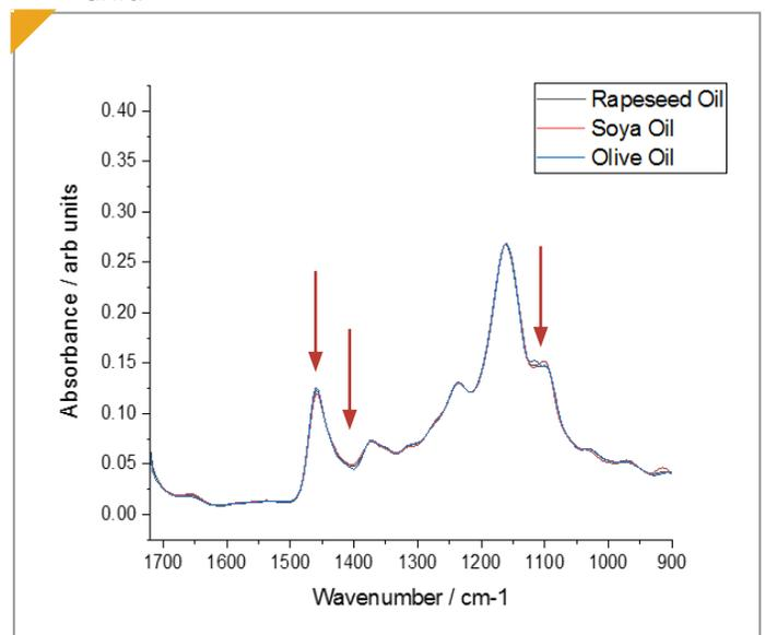
**Figure 1:** FTIR spectra of Rapeseed Oil, Soybean (Soya) Oil and Olive Oil as recorded by the IRmadillo Spectrometer with 120 s sampling time between 900 to 1740  $\text{cm}^{-1}$ . Key differentiating features are highlighted.
