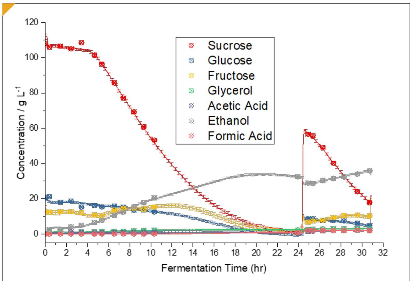
**Figure 1:** Plot of chemicals monitored by the IRmadillo during a fermentation process over 32 hrs clearly showing ability of the instrument to monitor multiple species simultaneously (sugars, acids, and alcohols).
