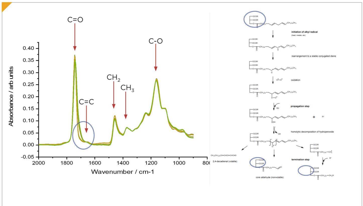
**Figure 2:** FTIR spectra of thermally degraded edible oil as recorded by the IRmadillo Spectrometer with 120 s sampling time between 900 to 2000 cm<sup>-1</sup>. The arrows show key peaks and intensities.
