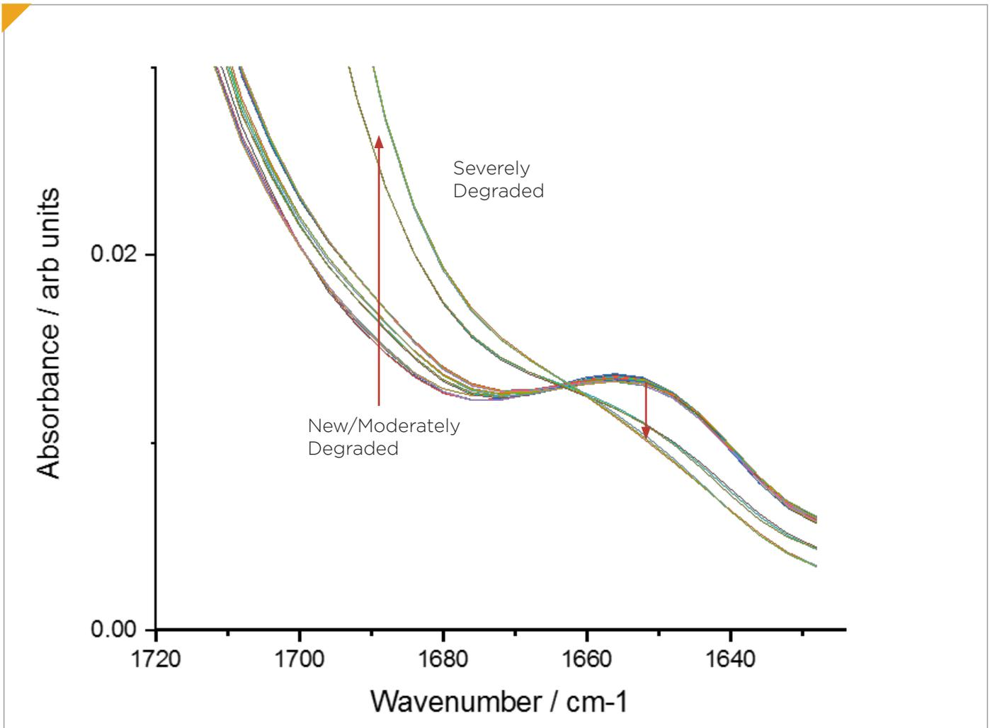
**Figure 3:** IRmadillo FTIR spectra of thermally degraded edible oil, isolating 1650 to 1720  $\text{cm}^{-1}$  to demonstrate the differences in analytical spectra depending on the level of thermal degradation and oxidation.
